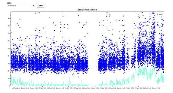
Select a date range, and click Load. Next select the loop you want to view data for and click view. The cyan line is the loop noise (Note: for TAG/Chronelec systems, the noise is only available for loops connected to the main decoder, not on remote decoders). The triangles are transponder passings and are coloured as follows:
